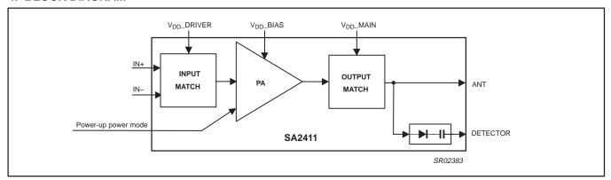
Figure 1. Block diagram
